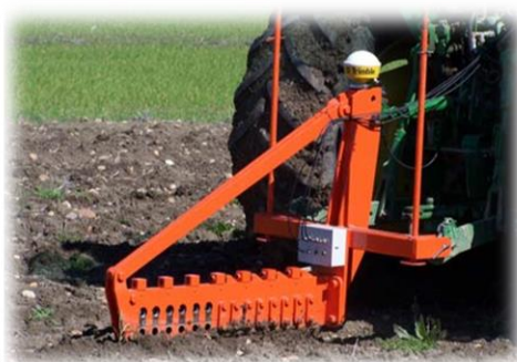
Figure 57: Source: Agüera, J.; Carballido, J.; Gil, J.; Gliever, C.J.; Perez-Ruiz, M. Design of a Soil Cutting Resistance Sensor for Application in Site-Specific Tillage. Sensors 2013, 13, 5945–5957.
