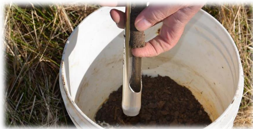
Figure 47: Traditional soil sampling (Source: https://www.indianaprairiefarmer.com/management/crops-consultant-prefers-soil-testing-management-zones )
