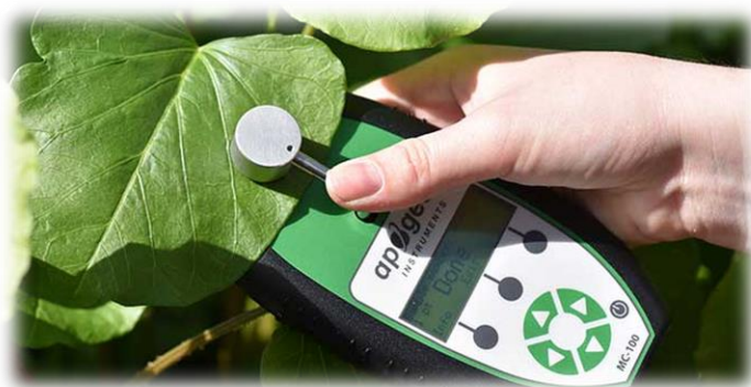
Figure 63: Chlorophyll measurement with chlorophyll content meter (Source: https://www.apogeeinstruments.com/applications-and-uses-of-chlorophyll-content-meters/ )
